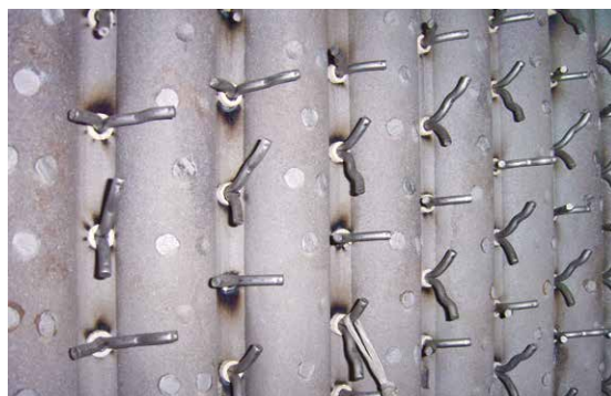
A wide range of geometries and anchor types can be welded as well as many different combinations of materials
